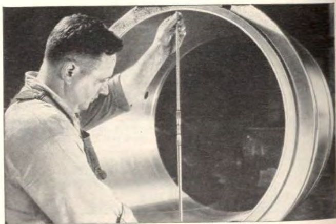
Using Inside Micrometer No. 681D, Built Up with Extension Rod at Both Ends
